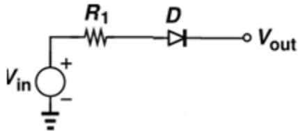
Q3. For the given circuit, what is the minimum peak value of the output waveform if the input waveform is 10V square wave with switching time of 1 second?
