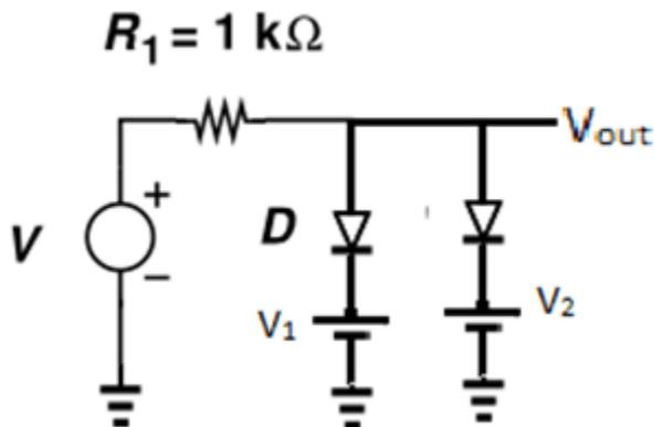
Q5. In the given circuit input voltage  $V_{in}$  is 3V and  $V_2$  is 1V. The resistance  $R_1$  is 1.5K. Cut-in voltage of diode is 0.5V. Forward bias resistance is  $10\Omega$ . The current  $I$  will be
